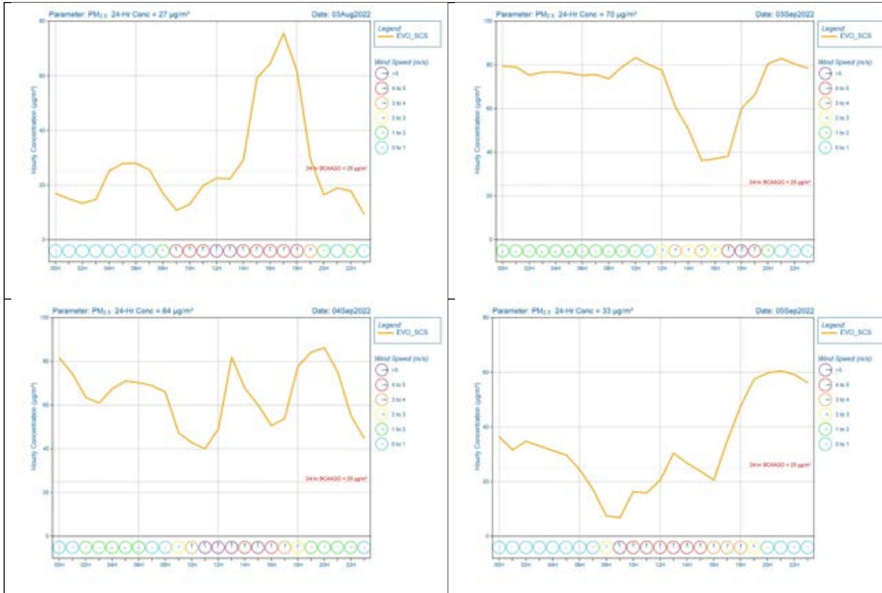
Figure C-2: Hourly winds and PM 2.5 concentrations at EV_SCS during days with excursions in 2022.
