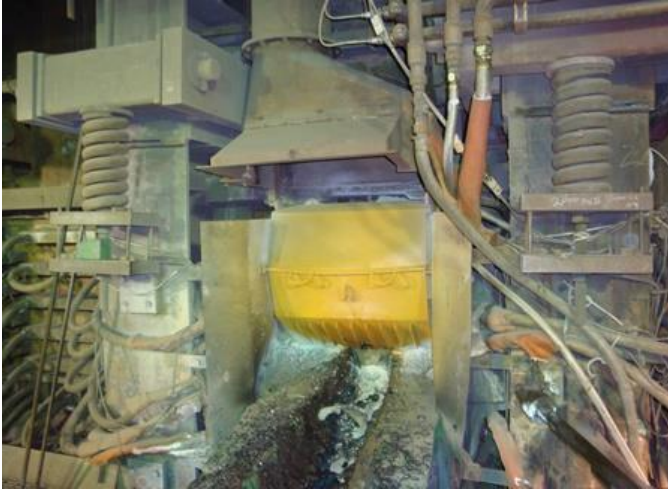
Figure 1. - Above: New collection hood on the Slag launder
