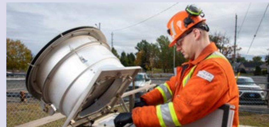
Adam May, Smelter Occupational Hygiene Technician, changing the particulate filter at the Air Monitoring Station in the town of Falconbridge.
